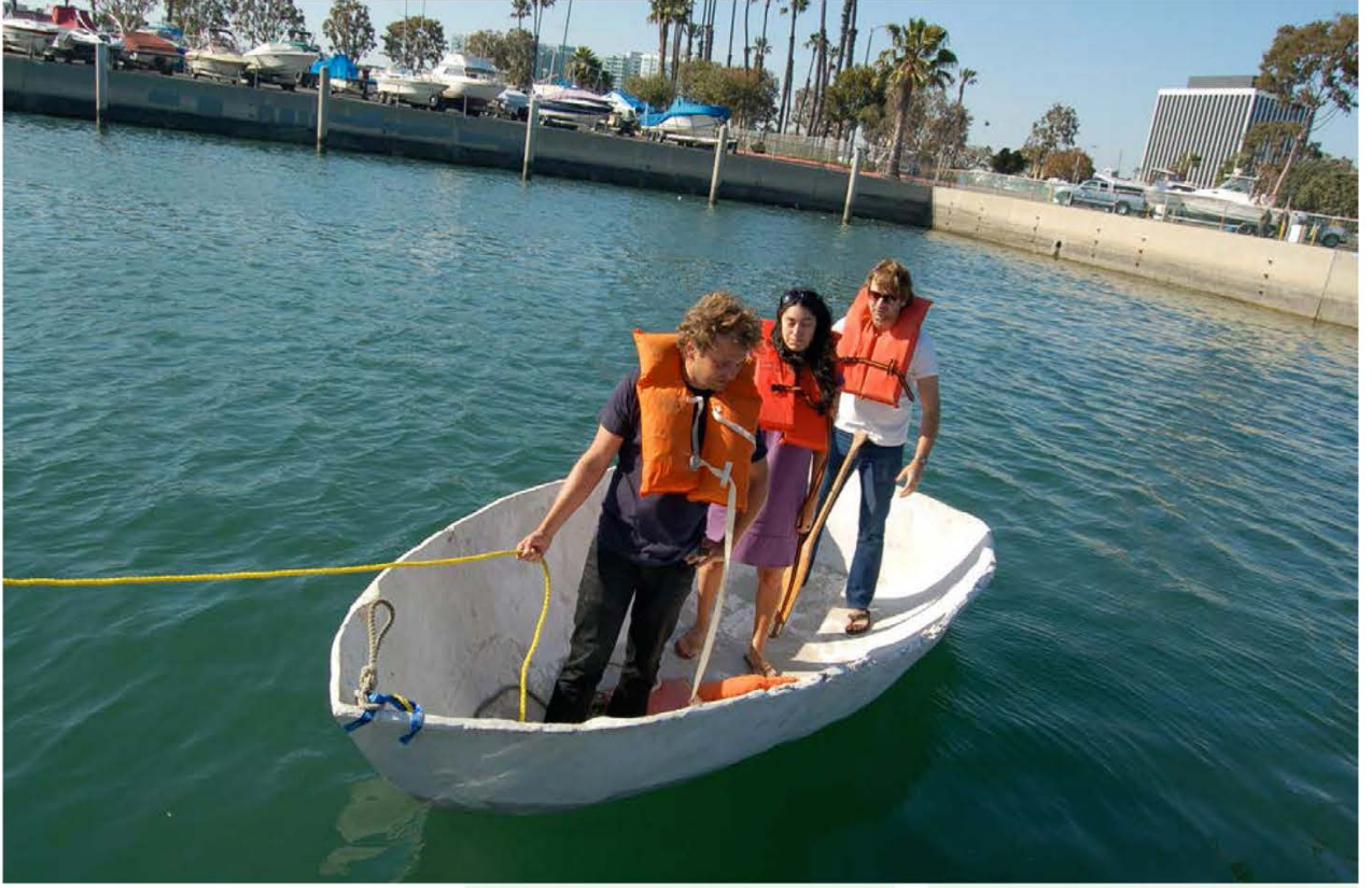
Brian O'Connell Concrete Boat Project [Beton Tekne Projesi] 2009 Portland betonu ve plaj kumu | Portland Cement and Beach Sand Los Angeles, CA yaklaşık 4x1.7x1.7 m.
