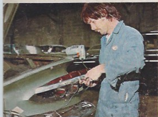
Work in progress: This is Garner making headlights out of tail-lights. Clips hold the lenses up so the Chevy can drive at night.
